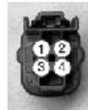
Air Fuel Sensor Wiring
